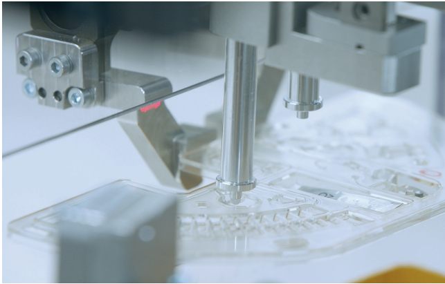
Here, a disk is filled with a spherical freeze-dried reagent (lyophilisate)
